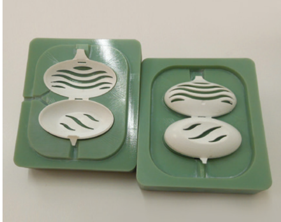
3D printed injection mold for a Domestic-brand toilet rim block
