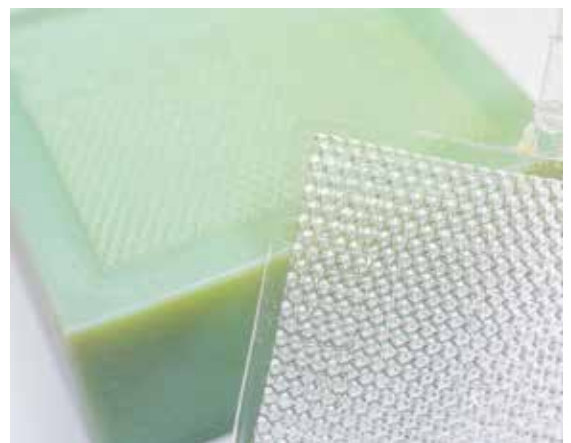
Injection molded prototype of LED headlight reflector that will be applied to metal backing to form finished piece
