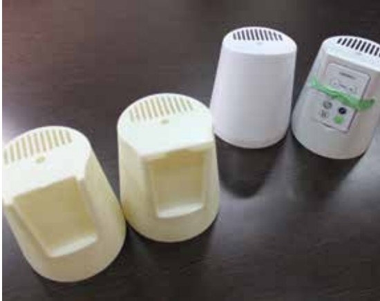
3D printed prototypes of the fan next to their finished counterparts
