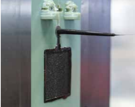
3D printed mold affixed to injection molding machine base
