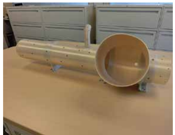
3D printed ECS duct with ULTEM 9085 material for its ability to withstand a wide range of extreme temperatures
